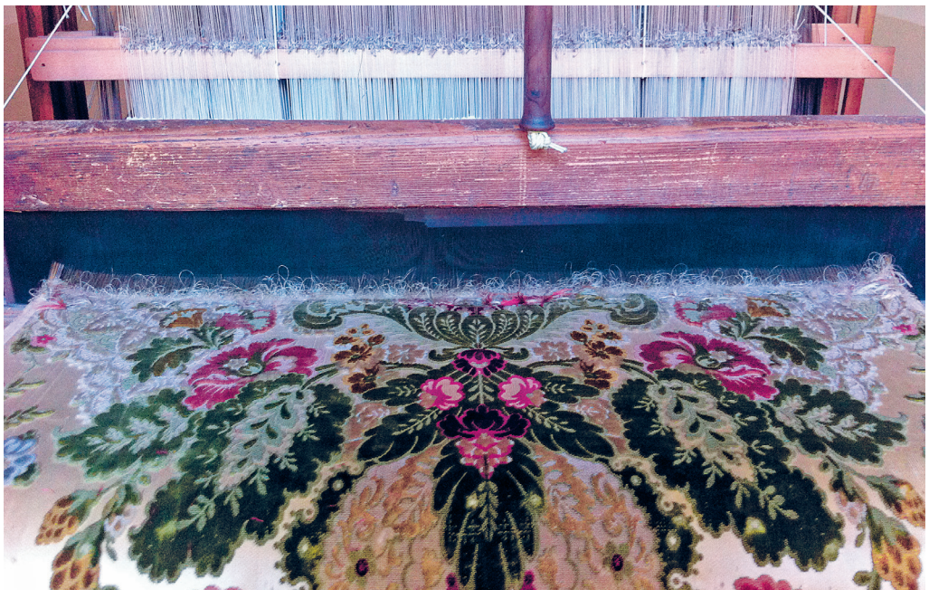
Figured velvet fabric, produced on historical Jacquard loom at the Fondazione Lisio, Florence. (Photo: Paula Hohti)
